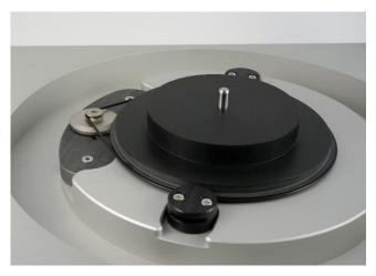
As a homage to the original EMT 928, the rotation power is transmitted by a belt. A most modern 20 Watts motor is combined with a high-precision control loop circuit in a compact assembly, to ensure short signal paths and to minimize interference. This design allows to speed up the 5,5kg platter in a short time and keep the platter speed constant within a narrow tolerance-field.
